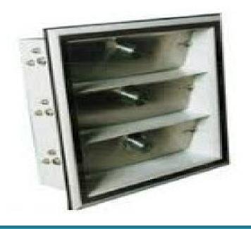
Pressure Relief Dampers should be provided in each room to prevent contamination of air from clean and dirty areas. Suitably sized air pressure relief damper should be strategically placed, enabling differential room pressure to be maintained and ensure that when doors are opened between clean and dirty areas. Counter weight balancing system should be provided in the PRD to maintain positive pressure inside the operation room.
